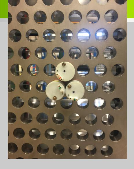
Rear View of 3 PMTs and bases installed in the shielding assembly
